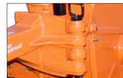
Foldable frame—for easy transportation when outside the field.
