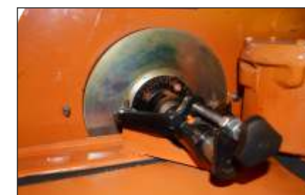
Inbuilt sharpening tool as a the standard fitment, helps sharpening the flywheel blades without removing them.
