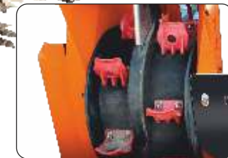
Cup Size suitable for 25 mm to 90 mm potatoes
