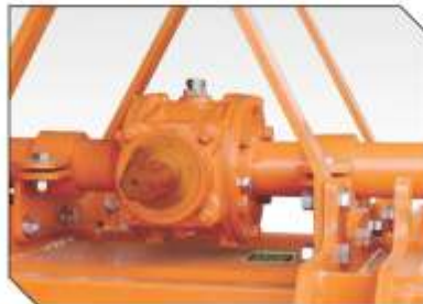
Specially designed gearbox for operation rotor in dual direction
